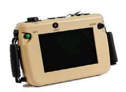
Designed for operators, the Brit-Vu is a compact Remote Viewing Terminal (RVT) that enables ground forces to receive video from airborne assets with C Band analogue data links. Brit-Vu receives imagery from airborne assets in real time giving the capability for ground forces to have an excellent situational awareness.
