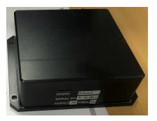
The 60004 Modem features high-performance dial-up modems designed for integration into a serial device through a MS38999 connector (others can be specified). The modem will automatically accept DC power inputs ranging from 16V to 40VDC and the supply is filtered to meet EMC requirements of RTCA DO-160. Data speeds from 2400bps, 14.4K, 33.6K to 56Kbps (V.92), and 14.4Kbs for fax.
